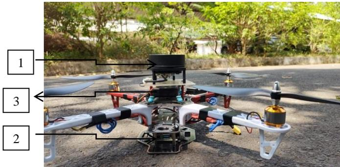
Fig-1: UAV system 1) LiDAR 2) Pixhawk 3) Raspberry Pi
